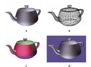
Changing the appearance of the 3D model A. Default appearance B. Wireframe rendering mode C. Colored lighting D. Different background color
